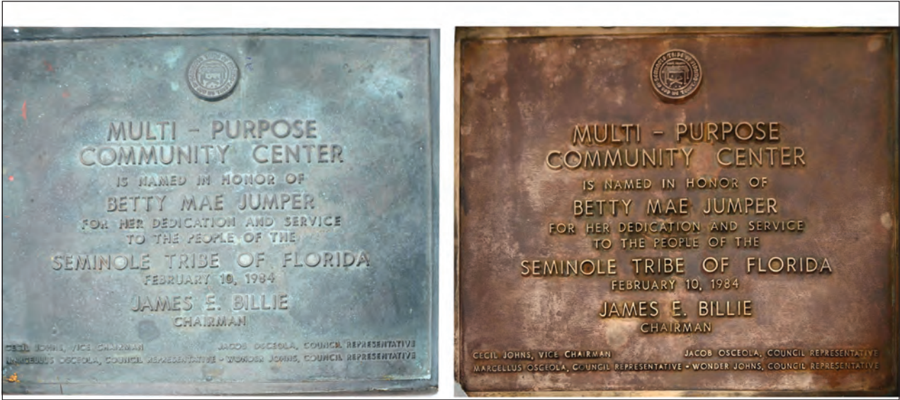
Ah-Tah-Thi-Ki Museum Left, bronze plaque before conservation treatment in 2020 with greenish blue corrosion. Right, the same plaque in 2025 after several rounds of mechanical and chemical cleaning to remove corrosion.
